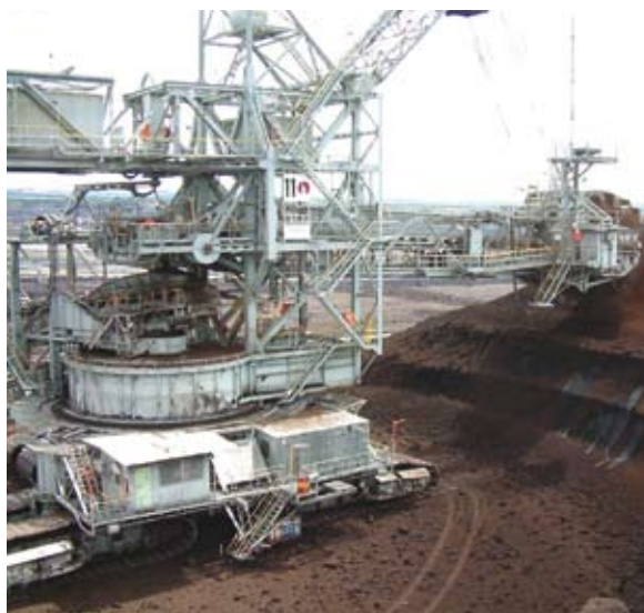
Hazelwood Mine, Australia Protected by Barrier and Jotamastic 87
