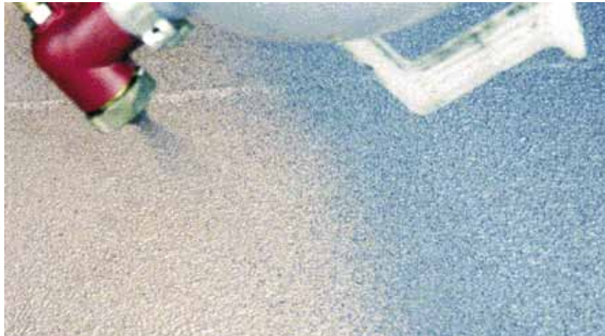
6. Application – circular motion should be used
